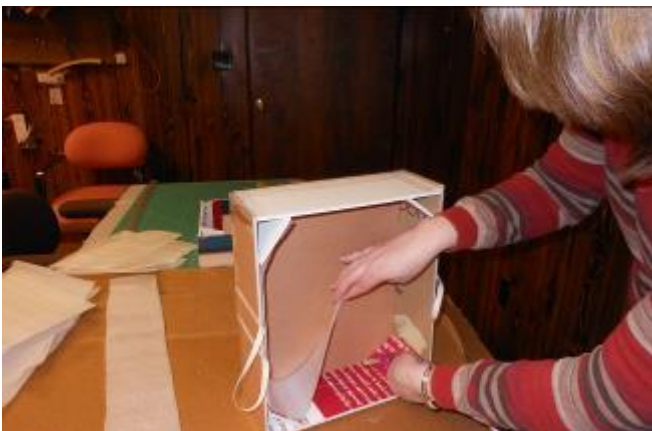
Divided trays for storage and transport from recycled materials. Applying foam sheets (left) and a finished tray (above)
